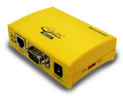
HD1320E can easily turn any RS232 serial device into a network device.
