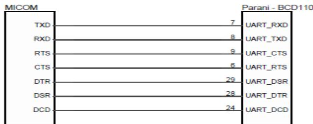
[ When TTL level of MICOM is 5.0V ]
