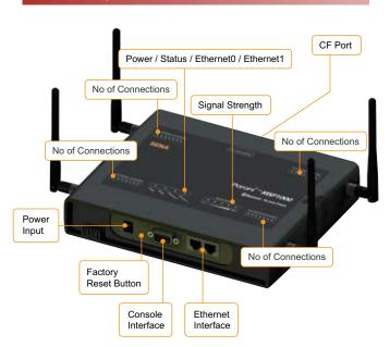
**The Parani-MSP1000** series is a Bluetooth Access Point to enable Bluetooth devices to be connected to 10/100Mbps Ethernet network. Parani-MSP1000 supports 7, 14, and 28 Bluetooth connections according to the model, and it supports up to 3Mbps throughput through Bluetooth 2.0+EDR specification. Parani-MSP1000 series is a class 1 Bluetooth device that supports 150m using basic dipole antenna and up to 1 km using patch antenna.
