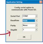
Parani-ESD Series default configuration is 9600 bps Baud rate, 8 Data bits, No Parity, 1 Stop bit and H/W flow control
