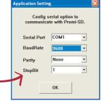
Parani-FSD Series default configuration is 9600 bps Baud rate. 8 Data bits. No Parity. 1 Stop bit and H/W flow control
