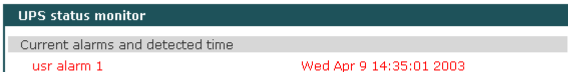
Figure 4- 1 User defined alarm is set
