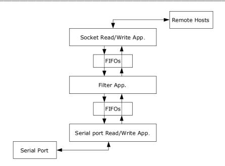
The user-defined filter reads a FIFO that is streaming the serial port data, manipulate the data and write the manipulated data to a FIFO that is sent to socket. The data stream that goes from socket to serial port can be manipulated in the same way. It must be satisfactory for following qualifications.
