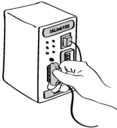
Figure 2-6. Connecting a serial console cable to the IALink100-Modbus
