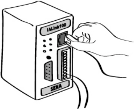
Figure 2-4. Connecting a network cable to the IALink100
