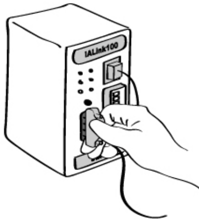
Figure 2-6. Connecting a serial console cable to the IALink100
