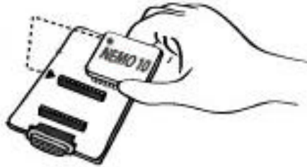
Figure 2-4. Installation of the NEMO10 module to the test bed
