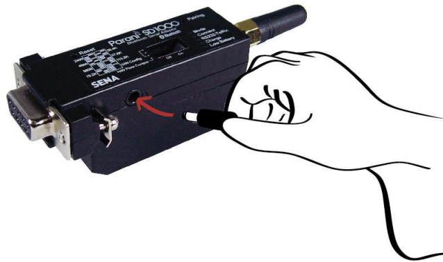
Figure 2-2 Connecting Power to Parani-SD1000
