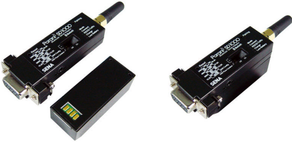
Figure 2-4 Attaching Batter Pack to Parani-SD1000
