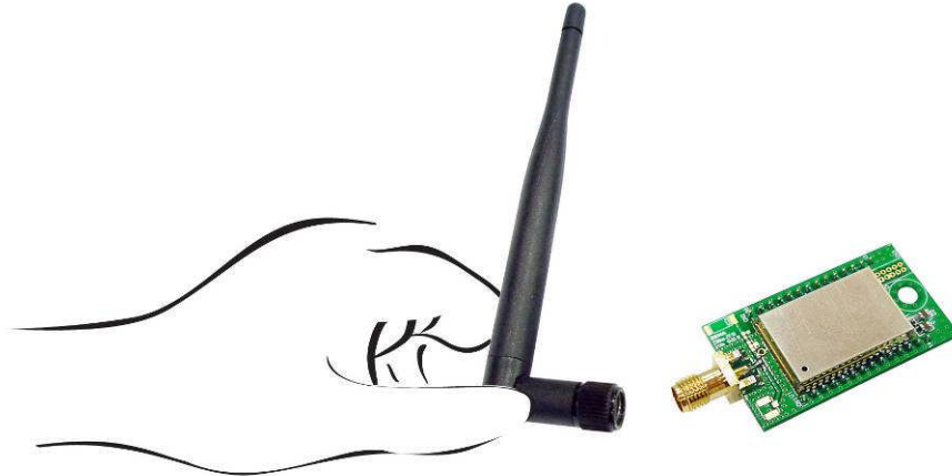
Figure 2-2 RP-SMA Dipole Antenna Installation
