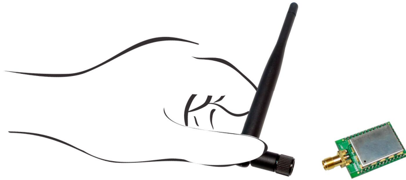
Figure 2-2 RP-SMA Dipole Antenna Installation
