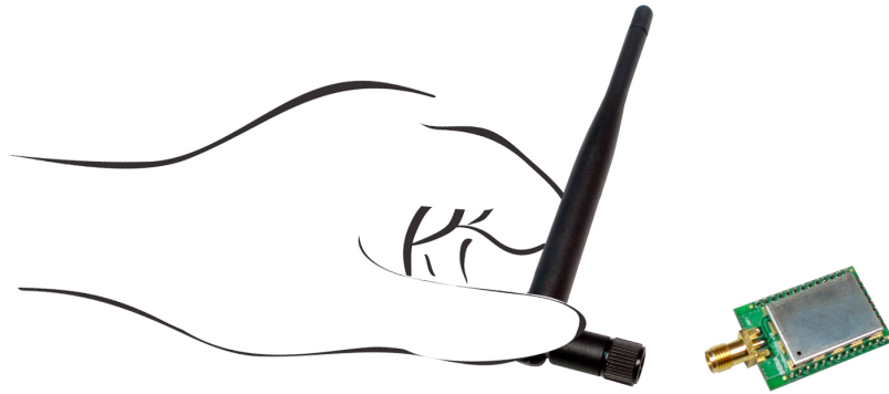
Figure 2-2 RP-SMA Dipole Antenna Installation
