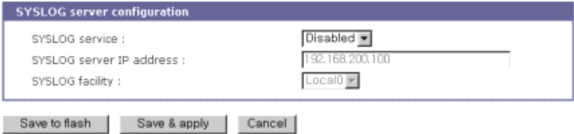
Figure 3-8 SYSLOG server configuration
