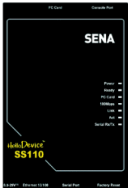
Figure 2-2 The panel layout of the SS110
