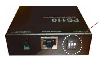
Set serial DIP switch according to your serial device requirements(RS-232/422/485)
