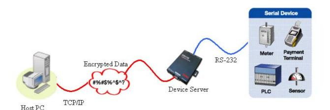
Basic application showing transport of encrypted serial device data over a plain view network by using a secure device server
